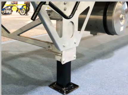
Integrated wing plate with reinforced K-bracing
