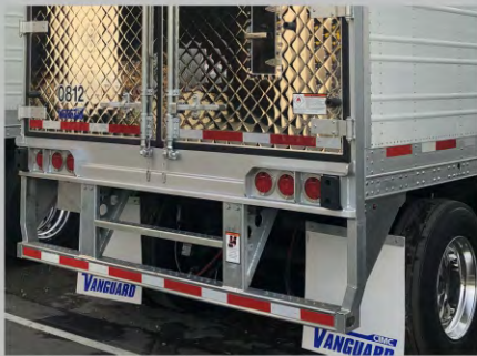
Hot dip galvanized rear bumper with outboard reinforcement
