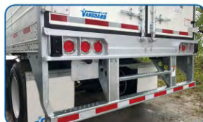
All galvanized bolt on structure with outboard reinforcement, strength exceed US DOT and Canadian DOT
