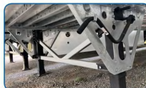
All galvanized bolt on landing gear assembly with integrated wing plate and reinforced K bracing to have better strength
