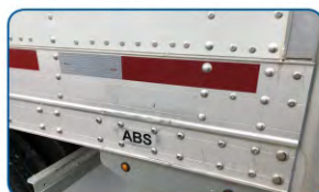
High base rail as standard for strong side wall structure
