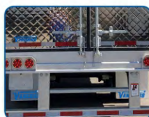
Integral lockrod with ATA structure to avoid pilferage
